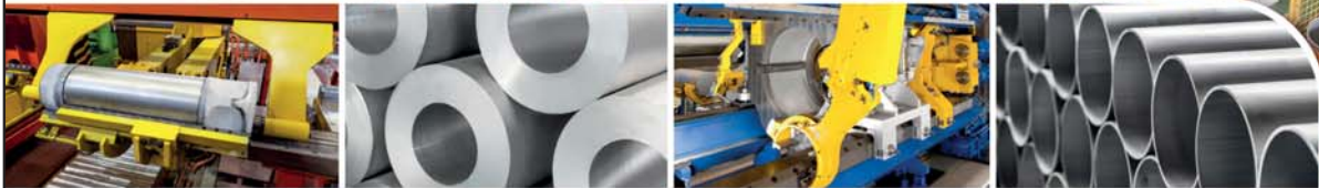
Jilin Liyuan, China; 45 MN Direct-Indirect-Tube Extrusion Press
