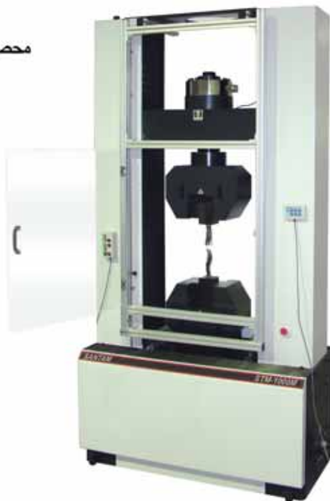
Universal Testing Machine Servo Electro-Mechanical Model 1000 kN Capacity
