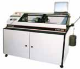
Torsion Testing Machine Servo Control Model 300 Nm Capacity
