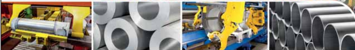
Jilin Liyuan, China; 45 MN Direct-Indirect-Tube Extrusion Press
