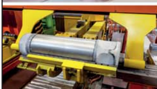
Jilin Liyuan, China; 45 MN Direct-Indirect-Tube Extrusion Press
