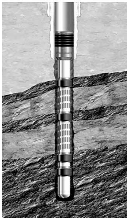
Figure (10). Use of swell packer to reach high production
