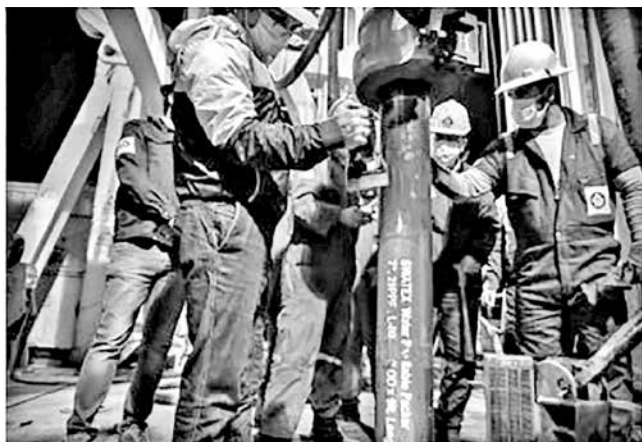
Figure (13). The 1st 7' 5ft. Long water Swell packer RIH successfully in Iran (Azar oil field)
